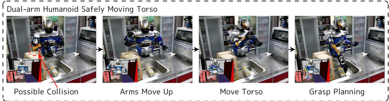
**Figure 3.16:** The planner is also applied to moving the torso joints of the robot such that the arms do not hit anything.
