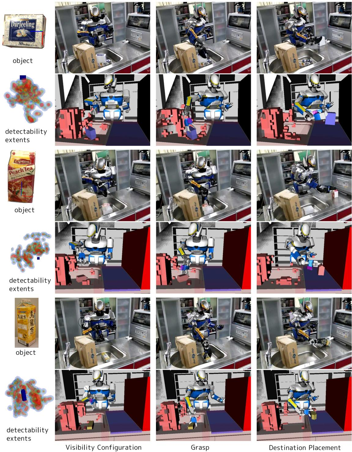
**Figure 5.11:** Manipulation with dynamic obstacles from range data (red boxes) using visibility configurations.
