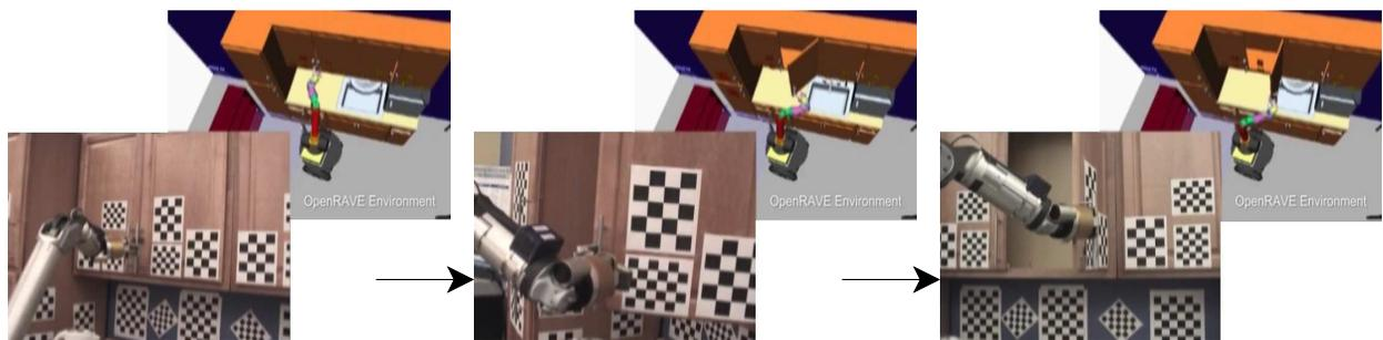
Opening a cupboard using hooking and pulling.
