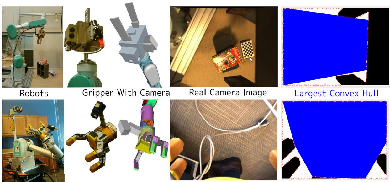
**Figure 5.3:** The real robots with the a close-up simulation of the wrist cameras are shown in the top two rows. Given the real camera image, the silhouette of the gripper (bottom) is extracted (black) and sampled (red), then the biggest convex polygon (blue) not intersecting the gripper mask is computed.
