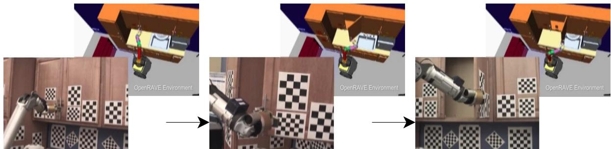
Opening a cupboard using hooking and pulling.
