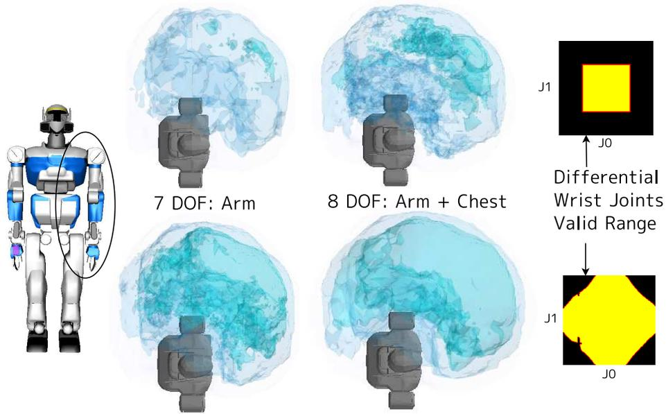
**Figure 4.19:** The HRP2 reachability space changes when the chest joint is added (left vs right). Also, the HRP2 wrist has a unique joint limits range, which can increase the reachability density by 2x if handled correctly.
